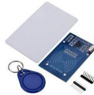
Fig. 4 RFID Reader and Tag
