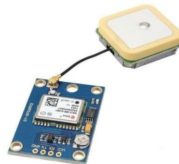
Fig.5 GPS Module NEO6M
