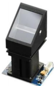
Fig.3 R305 Fingerprint Module
