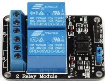
Fig.7 Relay module
